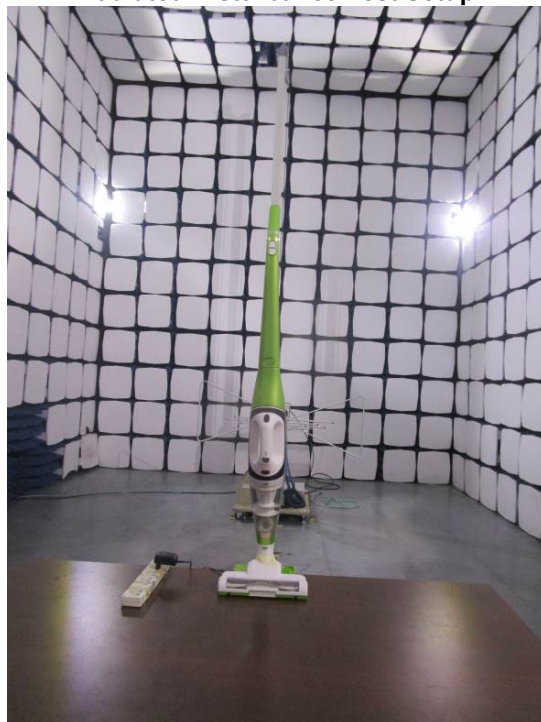
Radiated Disturbance Test Setup
