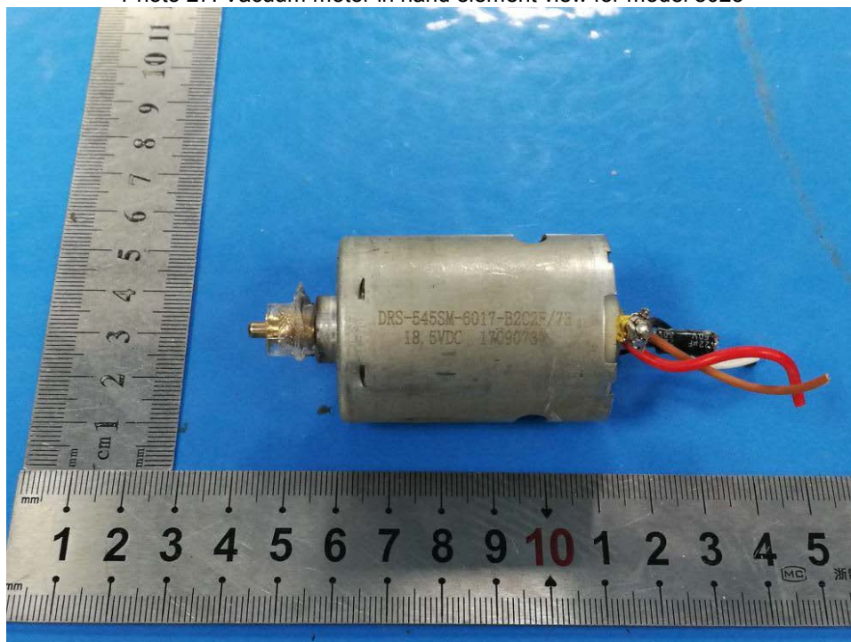
Photo 27: Vacuum motor in hand element view for model 8025
