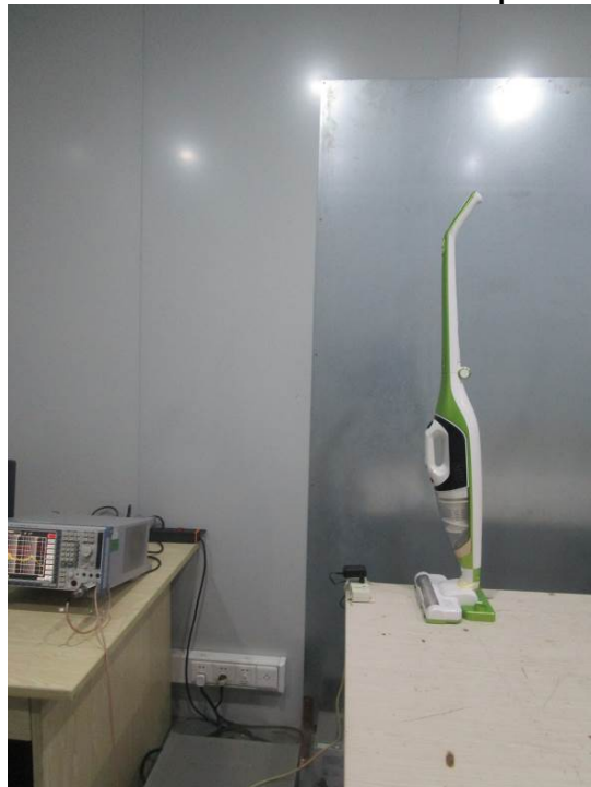
Conducted Emission Test Setup
