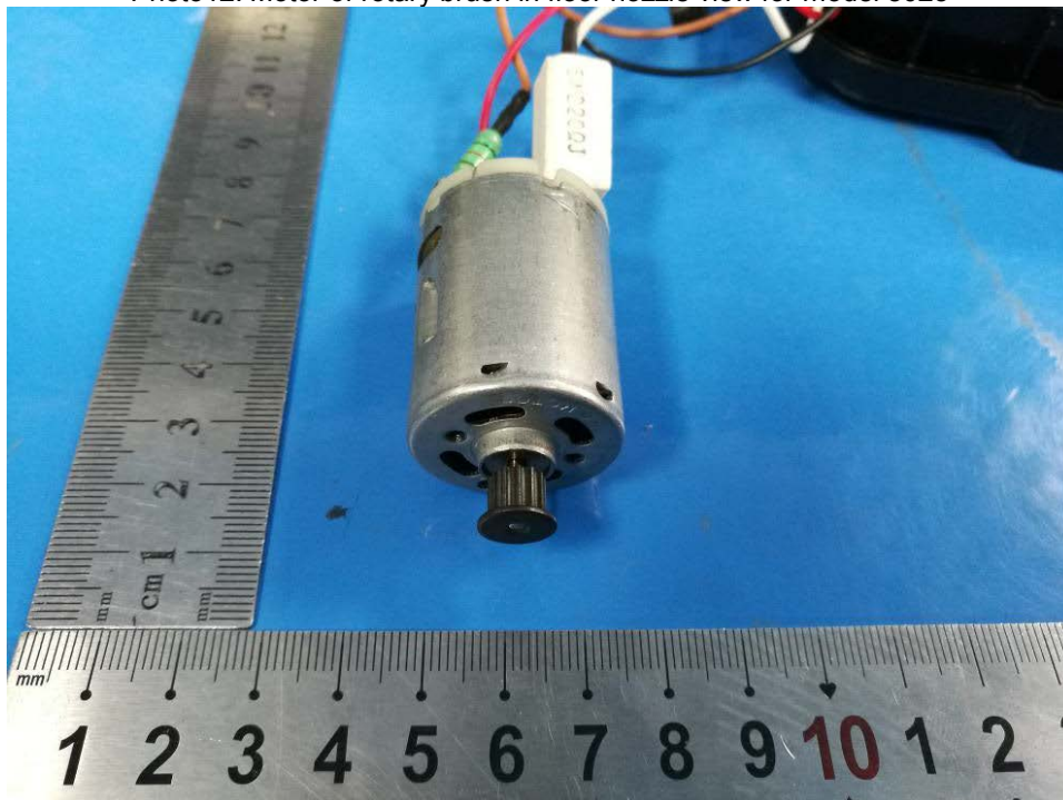
Photo12: Motor of rotary brush in floor nozzle view for model 8025
