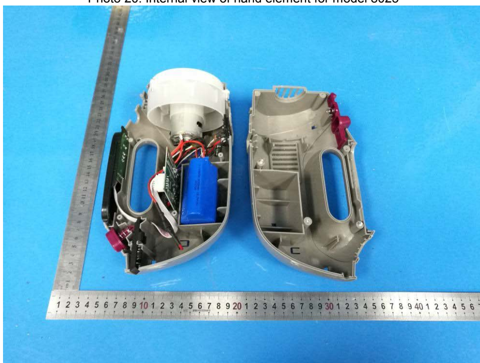
Photo 20: Internal view of hand element for model 8025
